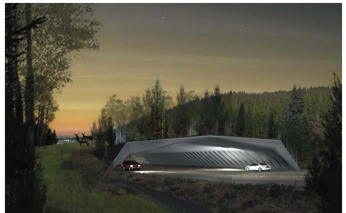
Graphic representation of the winning team's modular hypar vault system. One benefit of the design is that it isolates animals from road light and noise. (courtesy of HNTB and MVVA)
