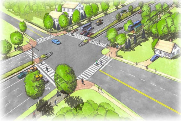
Ground-level and aerial schematics depict planned bicycle and pedestrian paths, green medians, and visible crosswalks along a 15-mile stretch of New York Route 347. (Courtesy of NYSDOT)
