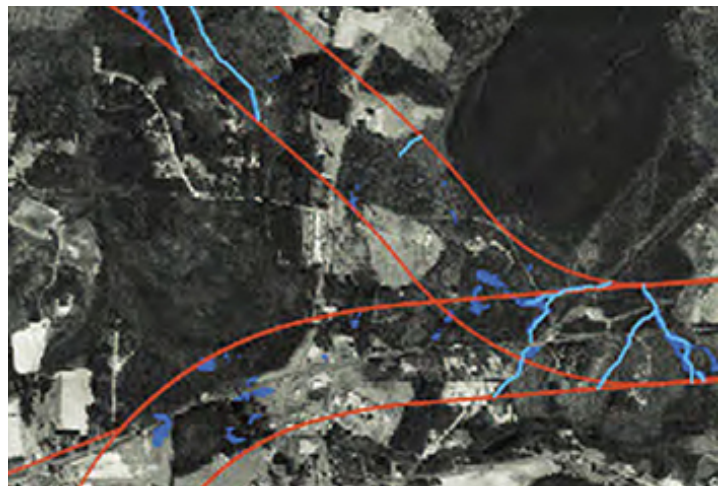
NCDOT and NCDWQ use LiDAR technology to develop maps such as this one to delineate wetlands and streams. (Courtesy of NCDOT)
