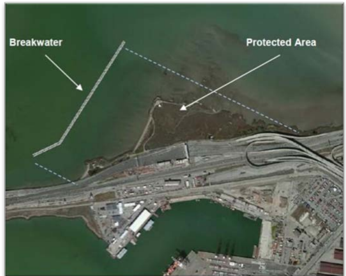
A breakwater placement and offshore configuration of Radio Beach, on the San Francisco Bay shoreline, would minimize wave action and overtopping of the levee as the sea level rises. (Courtesy of MTC)
